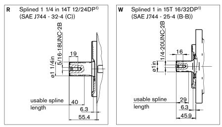
certifified installation drawing. Dimensions in mm
