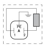
Plug connection to DIN EN 175301-803-A Cable screw joint M 16x1.5
