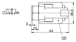
The female connector is not part of the scope of supply. This can be supplied by Rexroth on request.
