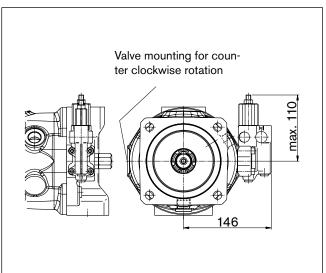
DRG - Pressure control, remotely operated
